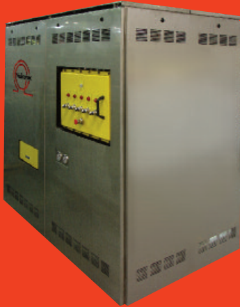
Vulcatherm® Heating / Cooling Thermal fluid : Water T° range : 20 / 110°C Heating Power : 30 kW (5 x 6 kW) ATEX Certified 6 separated controlled circuits
