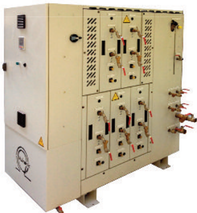
Vulcatherm® Heating / Cooling Thermal fluid : Water T° range : 20 / 140°C Heating Power : 50 kW (5 x 10 kW) 5 separated controlled circuits PLC controlled
